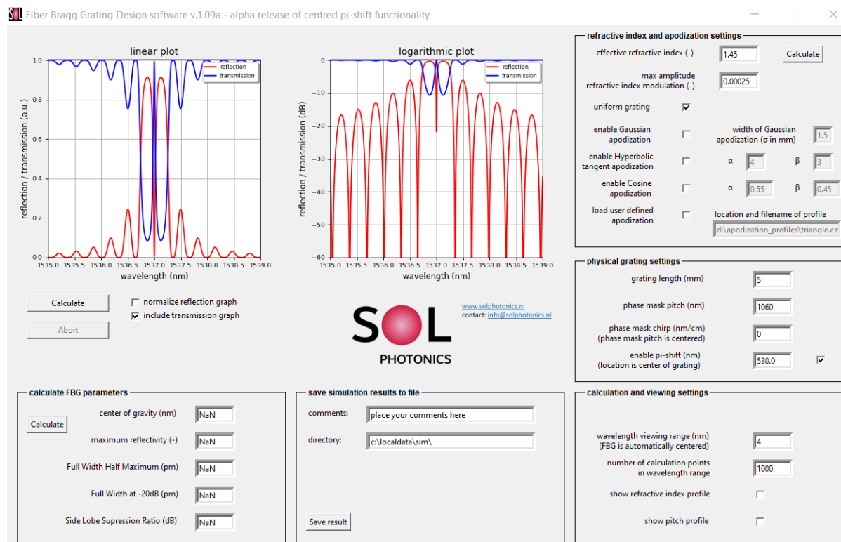
Figure 8: GUI of GDS including \pi -shifted grating functionality
